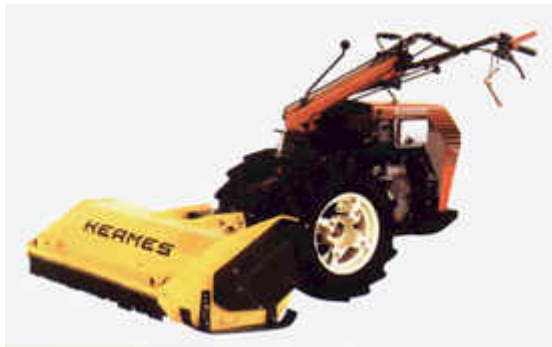
Photo 2. Hermes Flail Mower and walking tractor. Useful for removing crop residue, walking tractor $6000, flail mower $2200.
