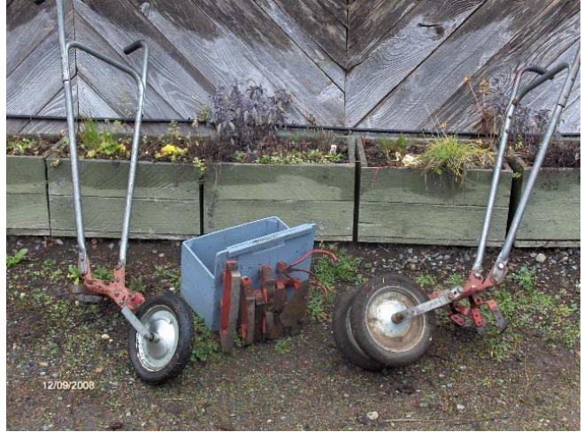
Photo 1. Glaser wheel hoe, one and two wheel configurations and various attachments Two wheel hoes $400 each plus $750 for tool set.
