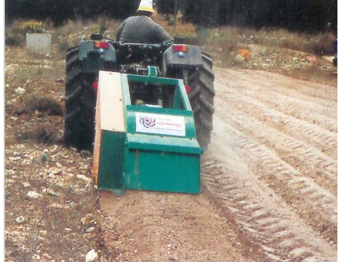
Photo 12. Agrimurge rock crusher requires 100 hp tractor. price $40,000.
